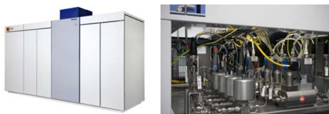
Figure: pictures of the Flowrence system with sixteen reactors
