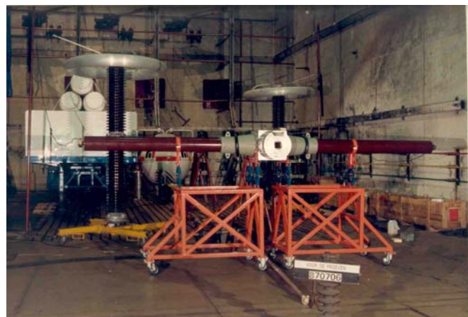
Figure 1 - Left: Submarine battery-powered short-circuit test facility operated by the Predecessor at Rotterdam Waalhaven (1984/87) - Right: Laval nozzle facility for its high-voltage breakdown tests at KEMA High-Power Laboratory (1986/87)
