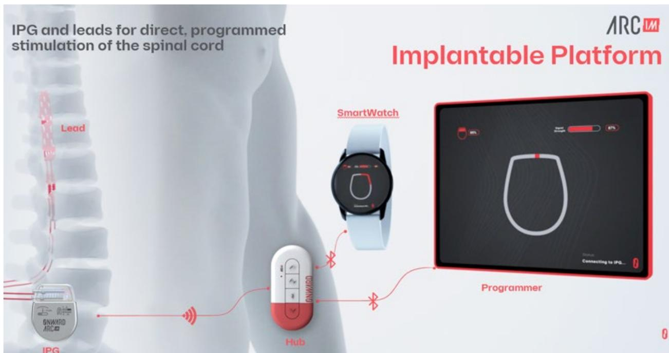
The IPG is controlled by a small, wireless external unit that is programmed and/or controlled by a tablet programmer or voice-activated smartwatch.
