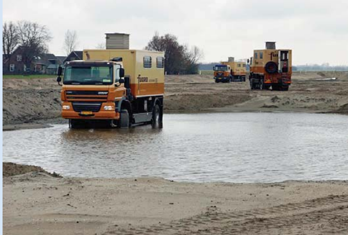
Fugro trucks performing cone penetration test, Delft-Schiedam, The Netherlands.
