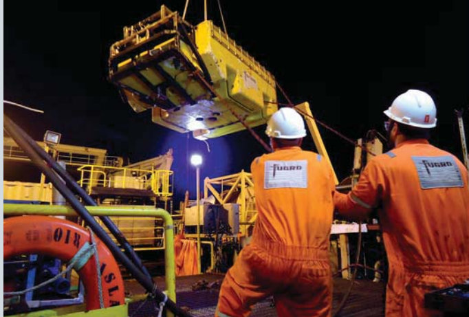
Recovery of a remotely operated vehicle (ROV) on board a ROV support vessel Island Spirit, Brazil.
