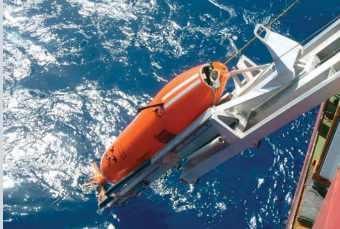
AUV deployment for seabed survey, Gulf of Mexico.
