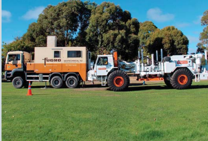
Fugro CPT truck collecting data for ground model analysis and design related to earthquake engineering, Christchurch, New Zealand.
