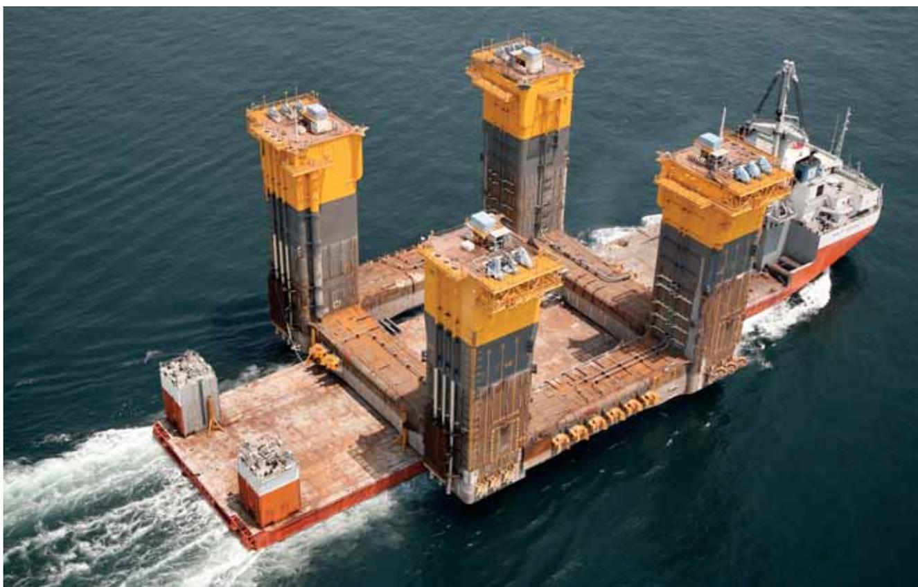
*The hull of the DeepDraft Semi™ floating production system for the Independence Hub during dry transport from Singapore to the Gulf of Mexico*
