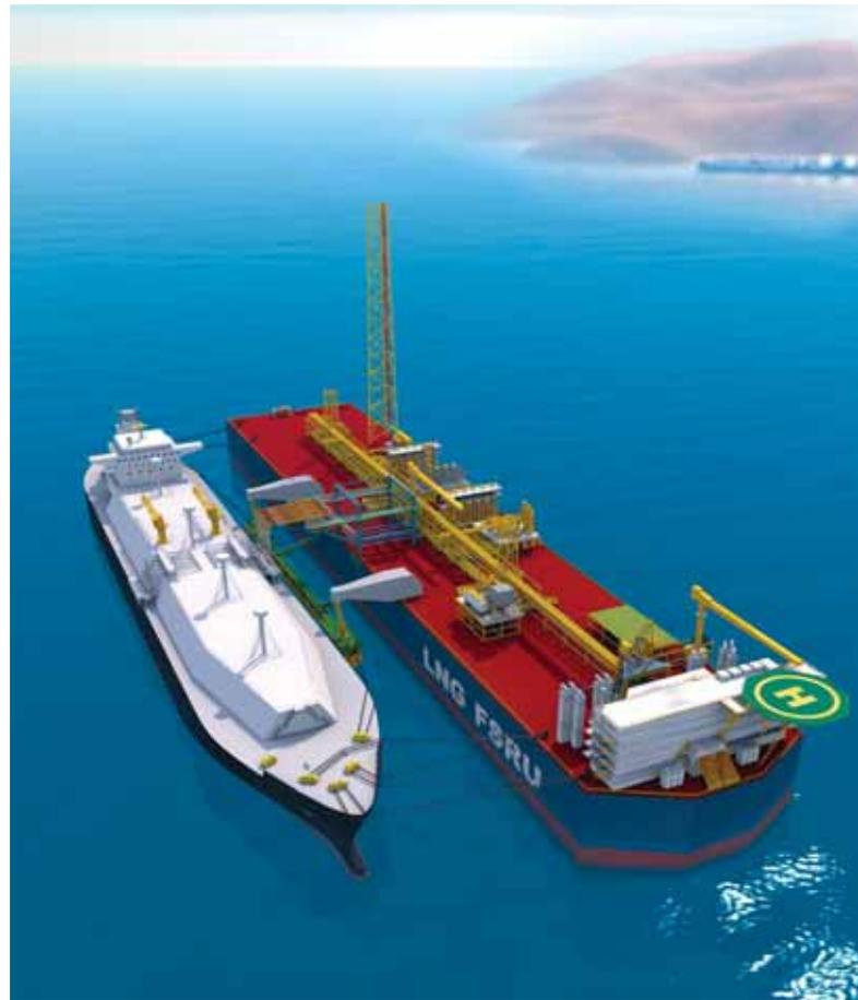
*Large capacity turret moored FSRU with a discharging LNG carrier berthed alongside on a Soft Quay Mooring*
