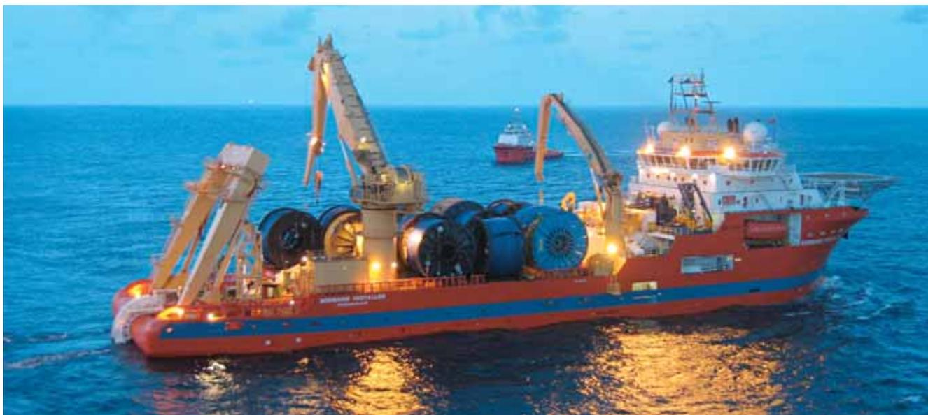
*'Normand Installer' during the installation of flexible flowlines at the Okwori field offshore Nigeria*
