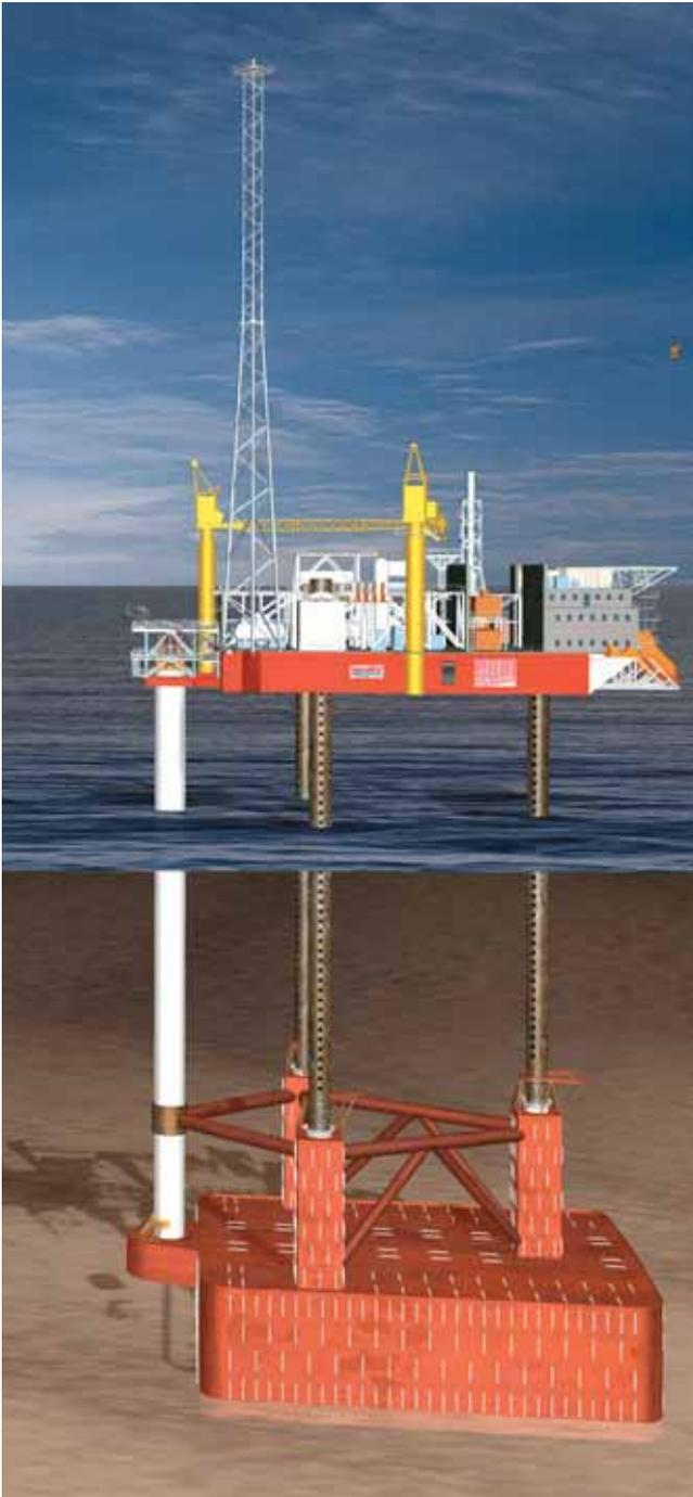
Computer generated image of the Mobile Offshore Production Unit with storage (MOPUstor™) for the Yme field offshore Norway; a lease contract for a new production concept in a new geographical area
