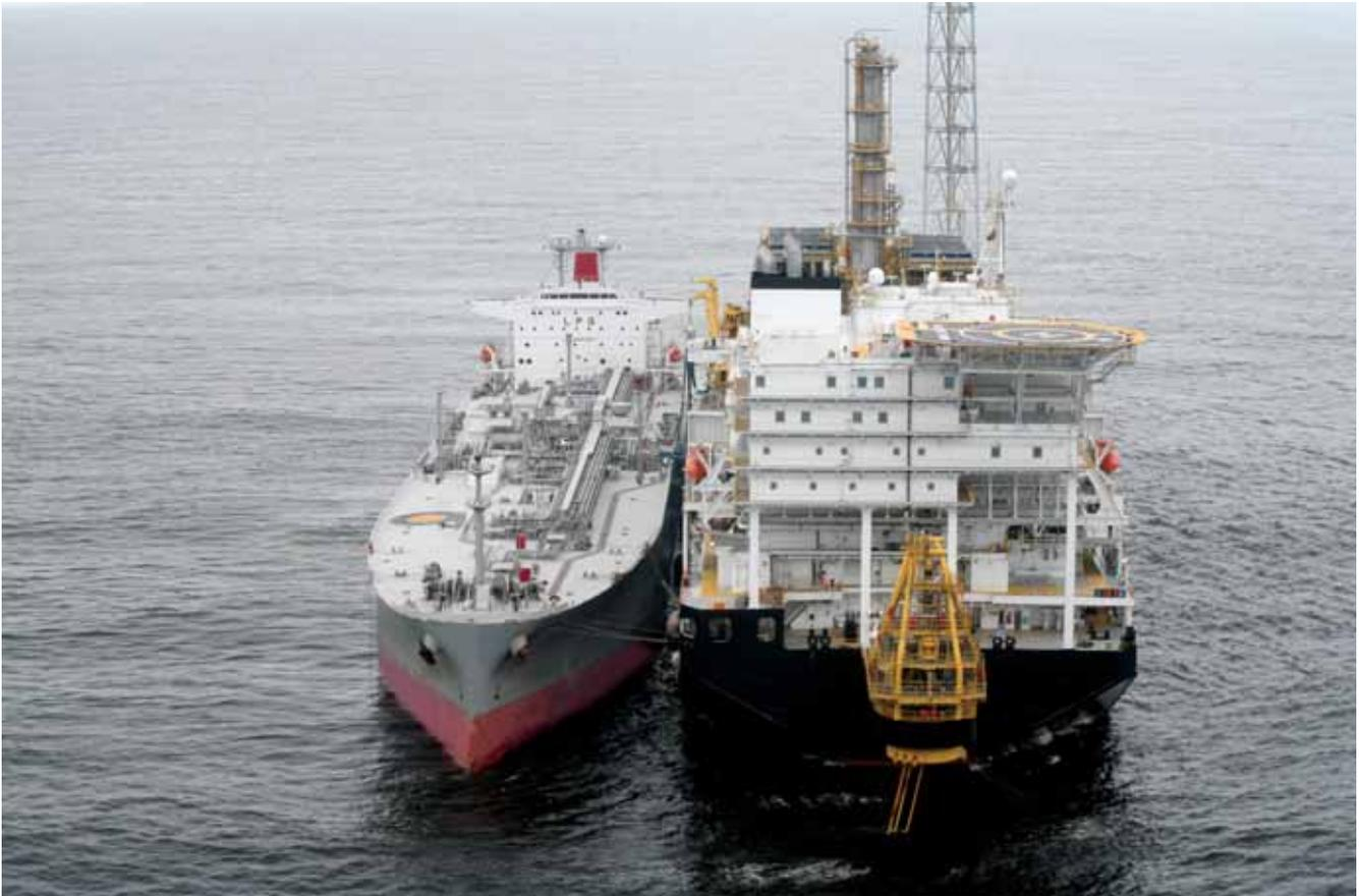
*Offloading of LPG from the Sanha LPG FPSO into an export tanker moored side-by-side*
