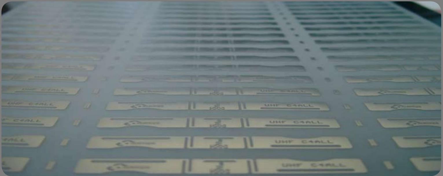
*Etched antenna production: SMARTRAC will enter the market of eTickets that require low cost etched antenna inlays in 2008*
