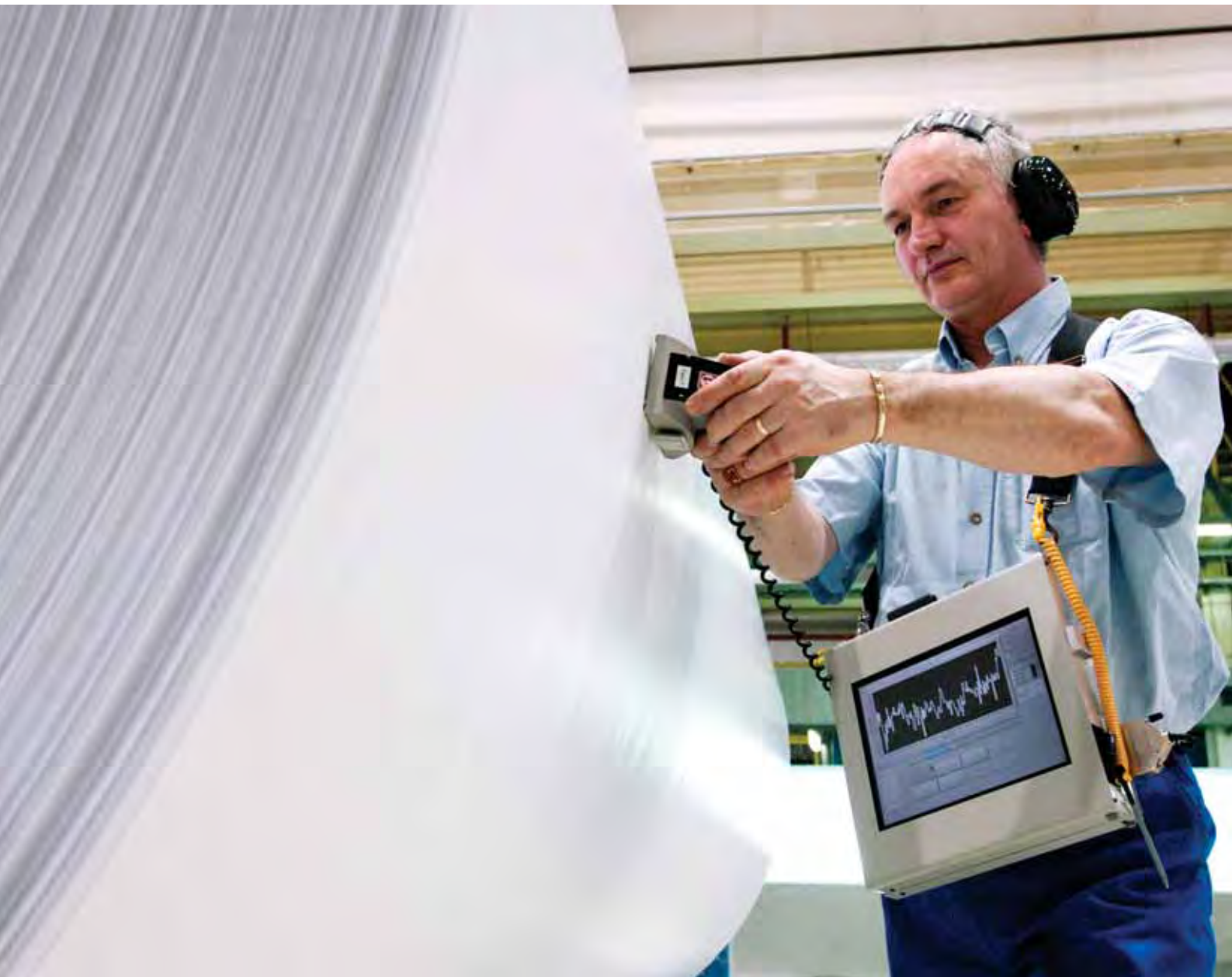
The measurement of reel hardness ensures better runnability at our customers.
