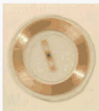
Wire transfer technology: Winded coils are placed on a substrate before lamination.
