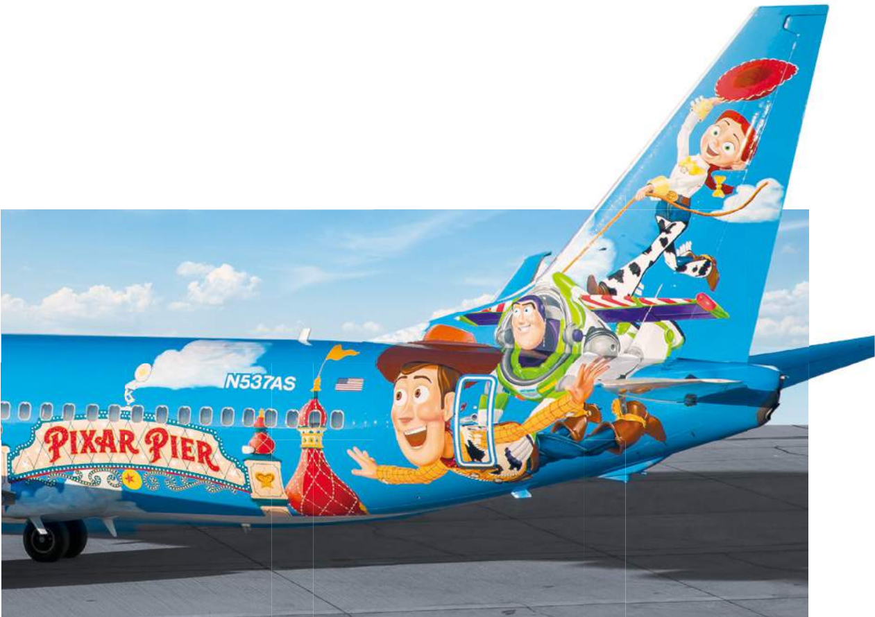
We helped Alaska Airlines to create a real buzz with special livery to celebrate the release of the movie Toy Story 4. We supplied our high-performance aerospace coatings for the specially themed plane, which took 24 days to coat and features 44 primary colors.
