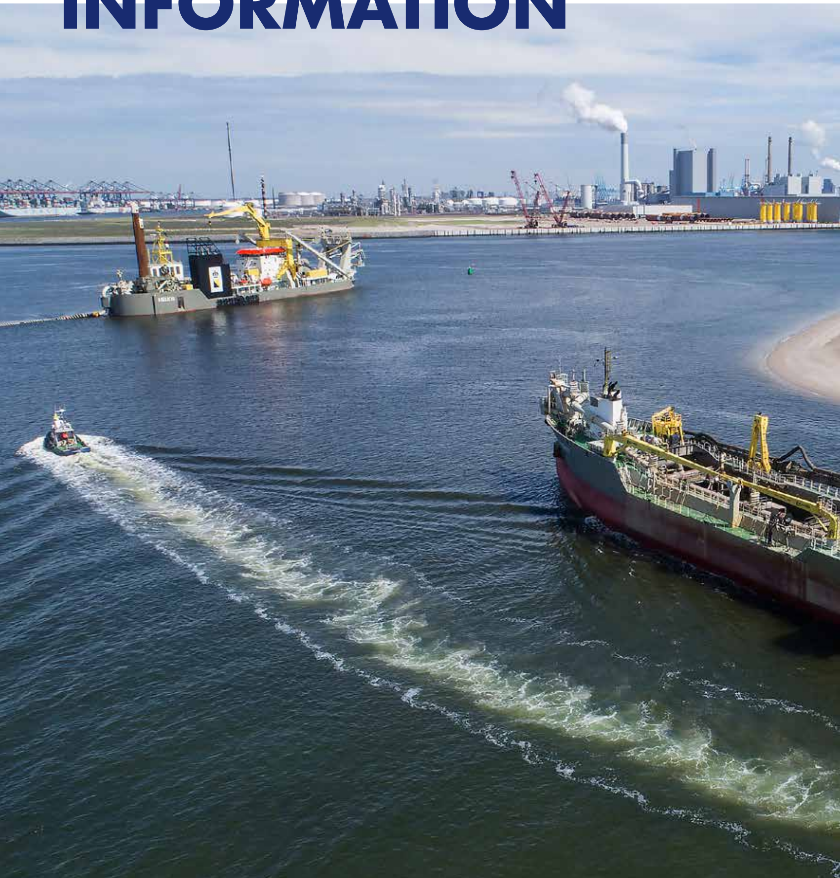
The mega cutter Helios and trailing suction hopper dredger Strandway dredging in the Port of Rotterdam.
