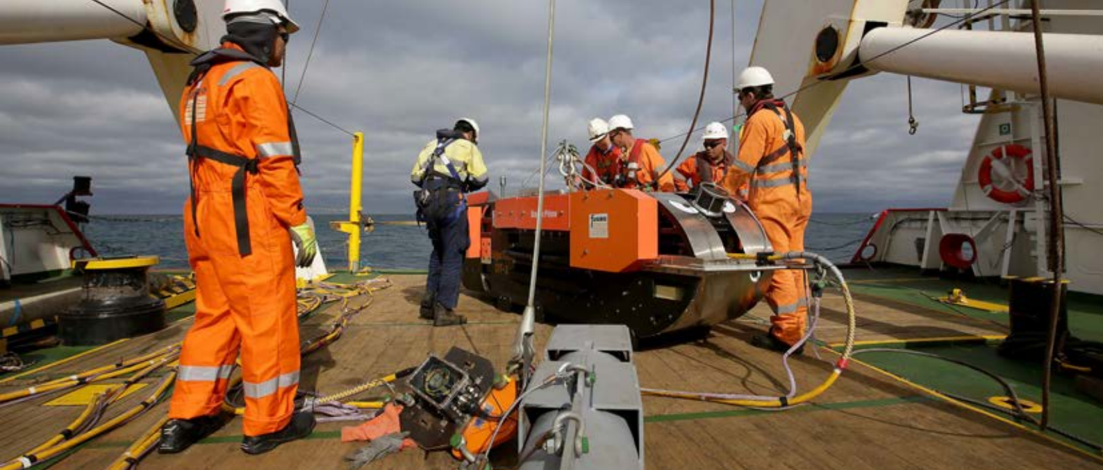
Fugro Discovery personnel prepare deep tow scanner in search for MH370 airplane.
