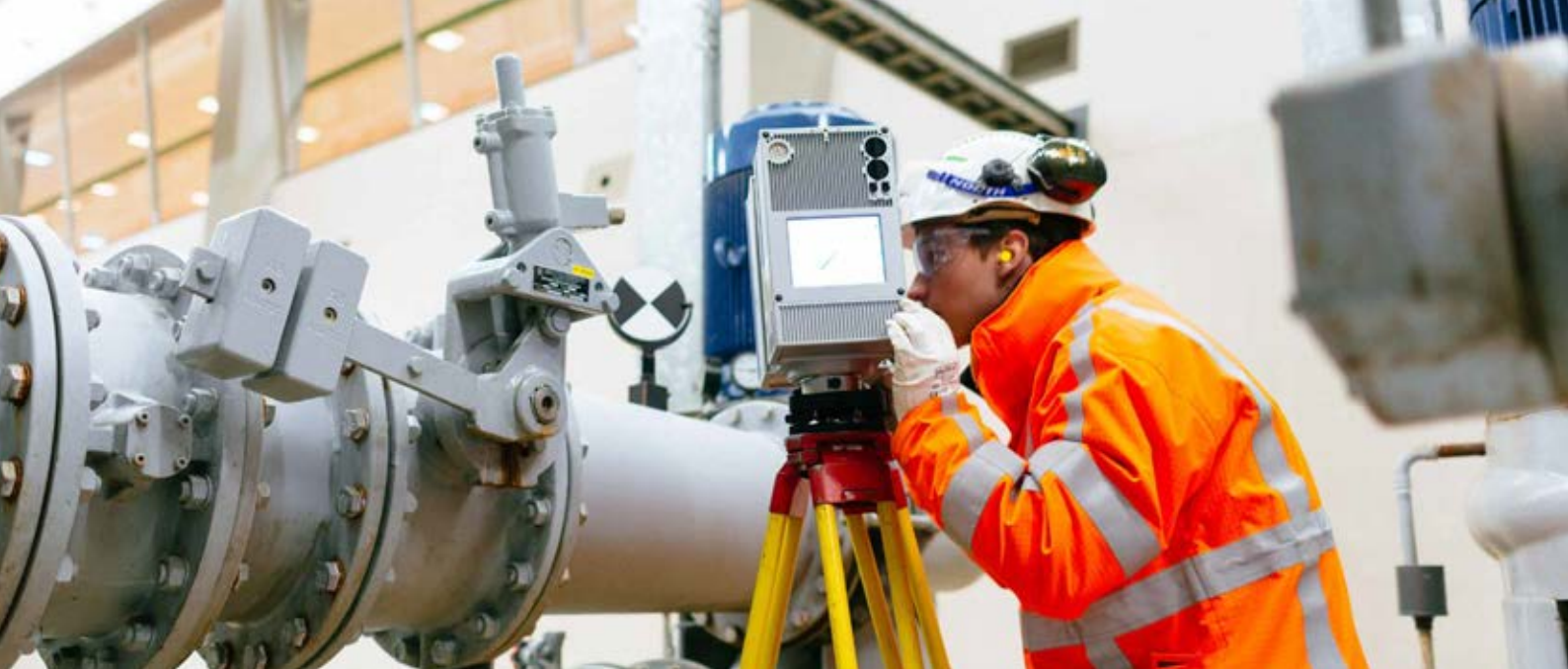
3D scanning of industrial installation, targeting efficient asset management.
