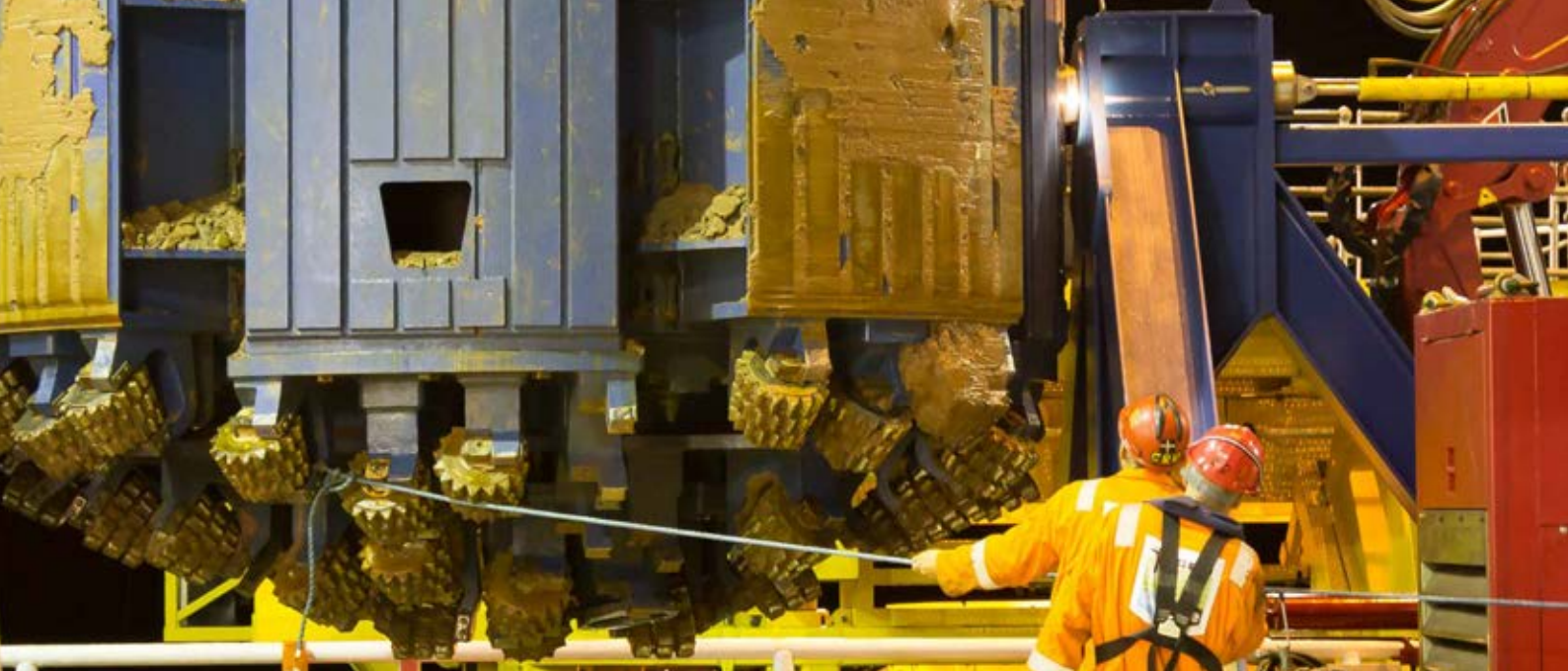
Drilling of large diameter vertical shafts.
