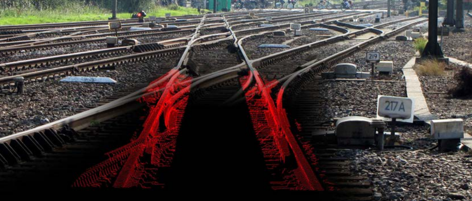
3D measurement of millimeters accurate track positions, to optimise rail safety and track management.
