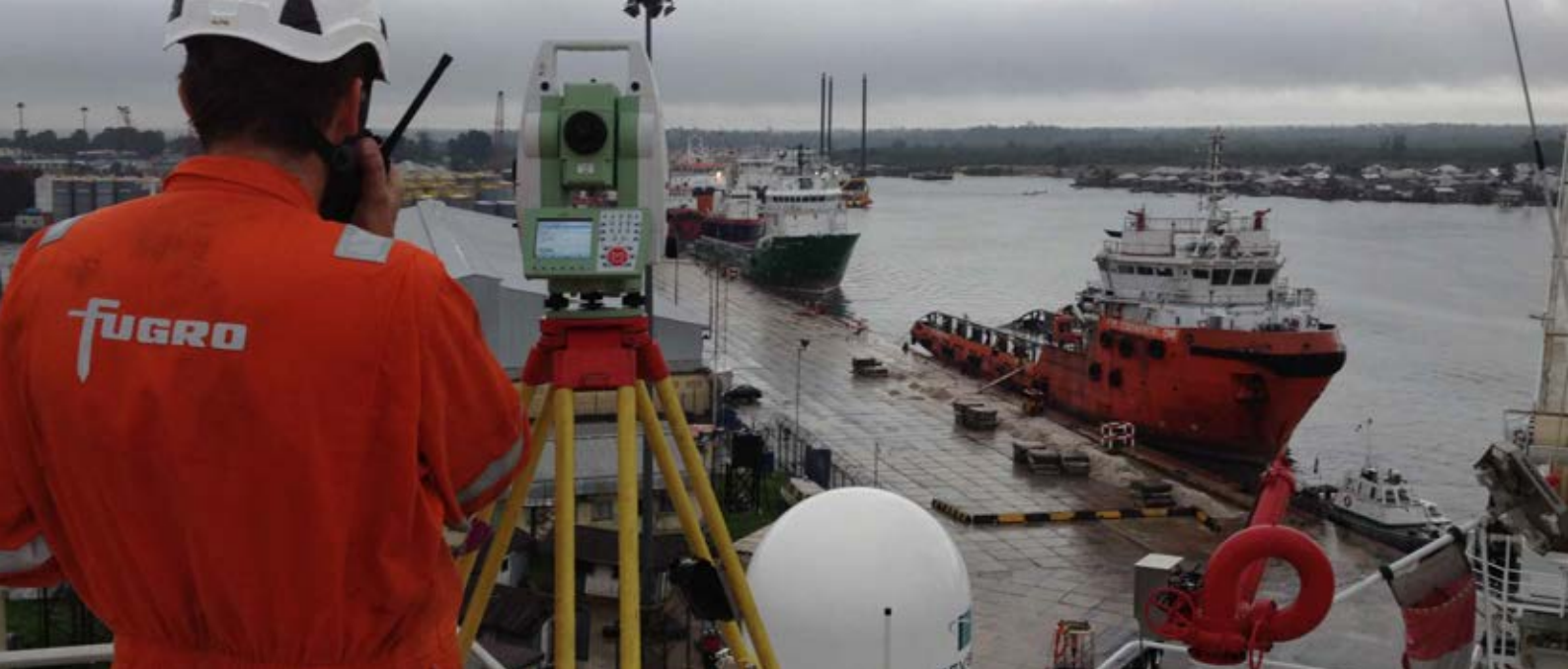
Calibration of vessels' instrumentation from quay side.
