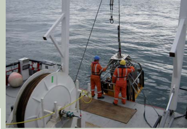
Conducting seabed CPT operations from the back deck of the MV Meridian
