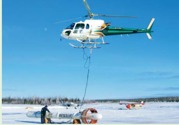
Electromagnetic airborne survey, High Lake Camp, Nunavut, Canada
