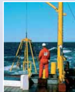
Launching "Searobin" for inspecting cable routes
