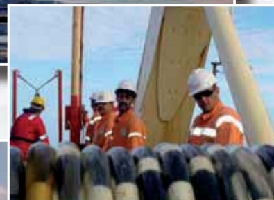
Rolling out streamers for a seismic survey in Western Australia
