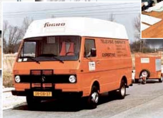
Fugro van for visual inspection of sewers and mains
