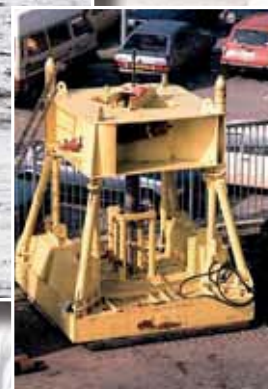
Seacalf for CPT tests
