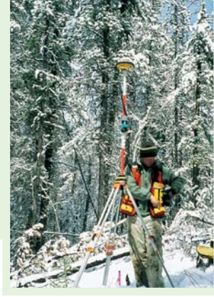
Surveyor with satellite positioning system, Rocky Mountains, Canada 2002
