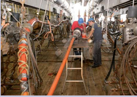
Streamer deployment onboard the seismic vessel 'Geo Atlantic' 2007
