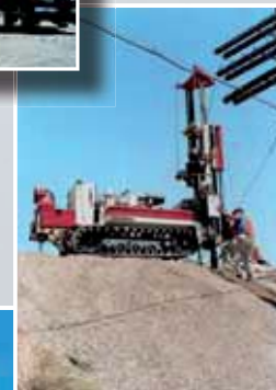
Taking soil samples near a railway in California
