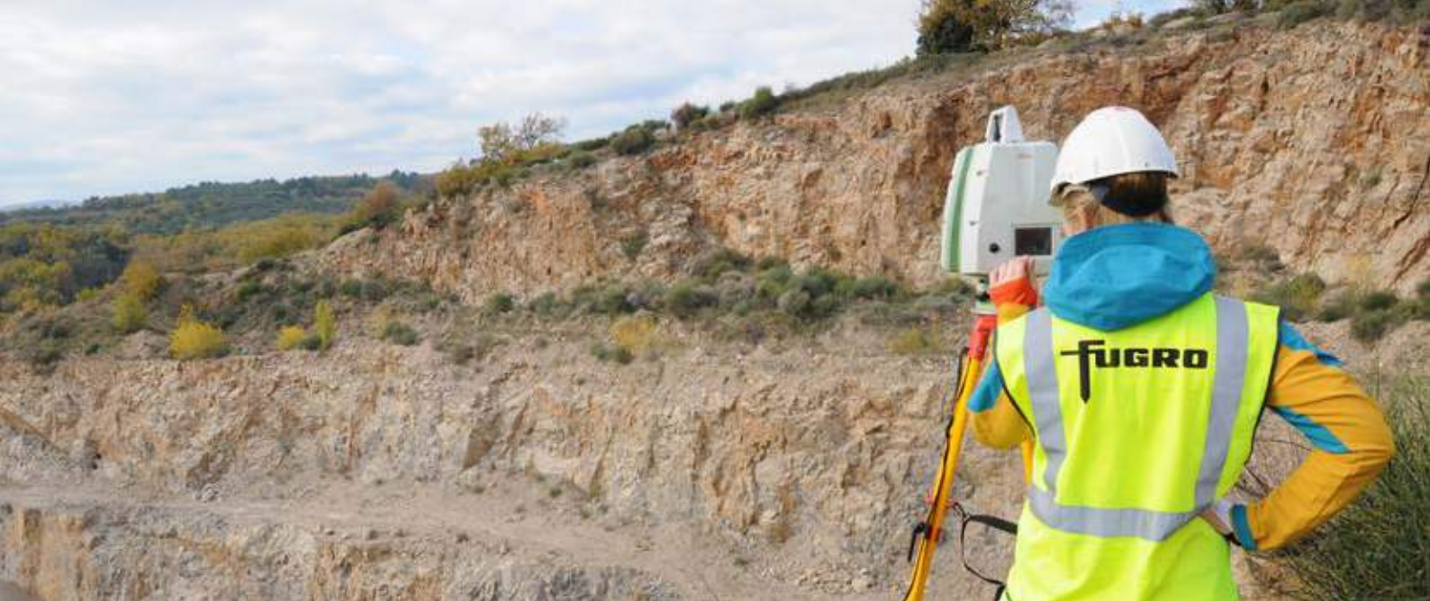
3D scanning of an op mining pit, Usclas du Bosc, France.
