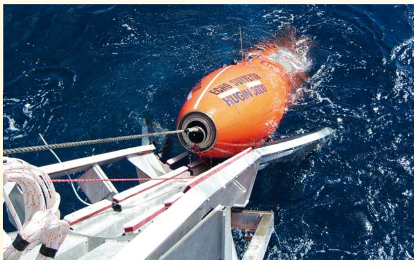
Recovery of an AUV (Autonomous Underwater Vehicle) in the Gulf of Mexico.
