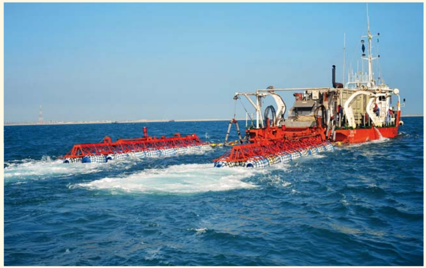
Airgun source deployment in shallow water, Arabian Gulf, Saudi Arabia. By courtesy of CGG and ARGAS, part of Seabed Geosolutions.
