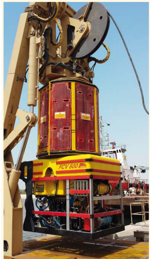
One of Fugro's ROVs undergoing wet tests from quay side in Abu Dhabi prior to a pipeline inspection campaign for Saudi ARAMCO, United Arab Emirates.
