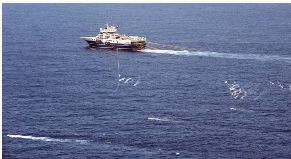
The Geo Caspian in acquisition mode offshore Tanzania with a 12 streamer spread operating and delivering high quality 3D seismic data.
