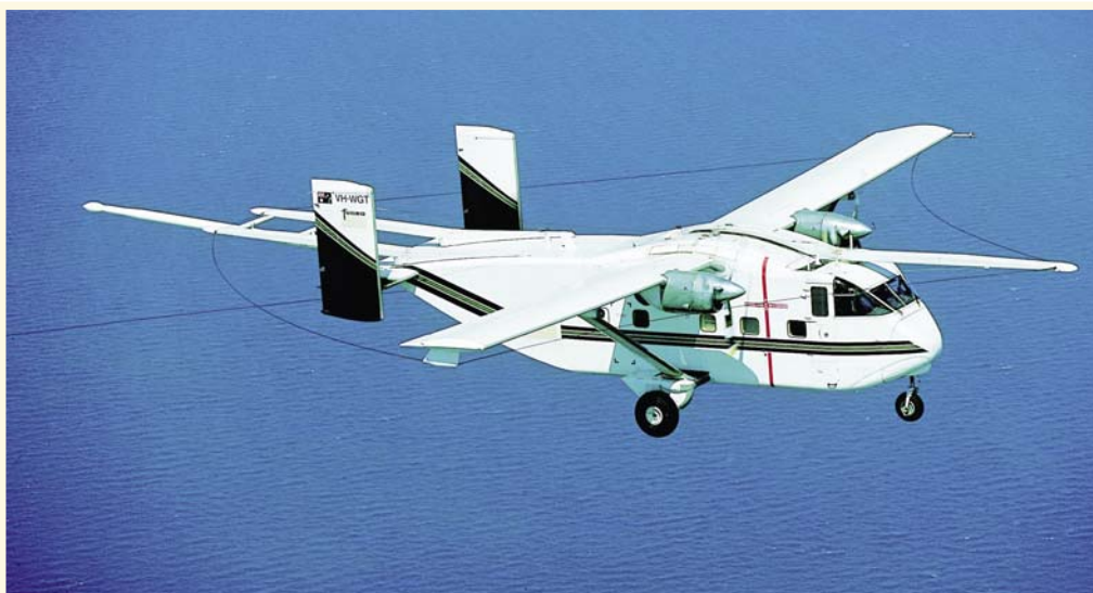
Airborne electromagnetic groundwater mapping, Australia.
