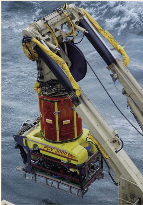
ROV in launching system.
