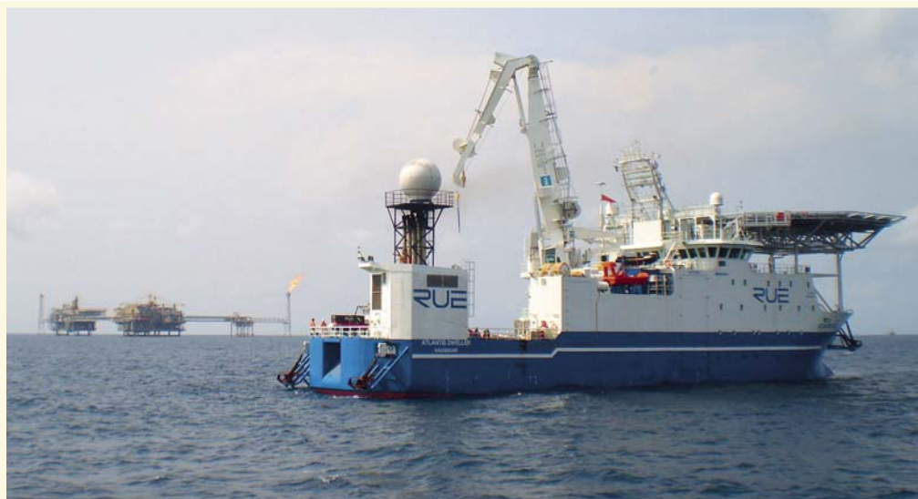
MPSV Atlantis Dweller off the coast of Nigeria for IRM work. The Atlantis Dweller is a multi purpose vessel designed to support diving and ROV.
