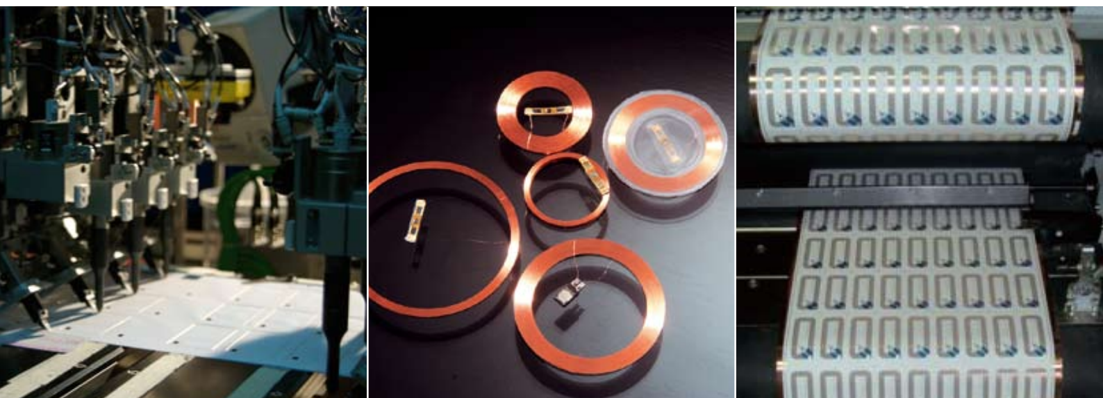
Leading edge antenna technology: wire-embedding, coil-winding and etching
