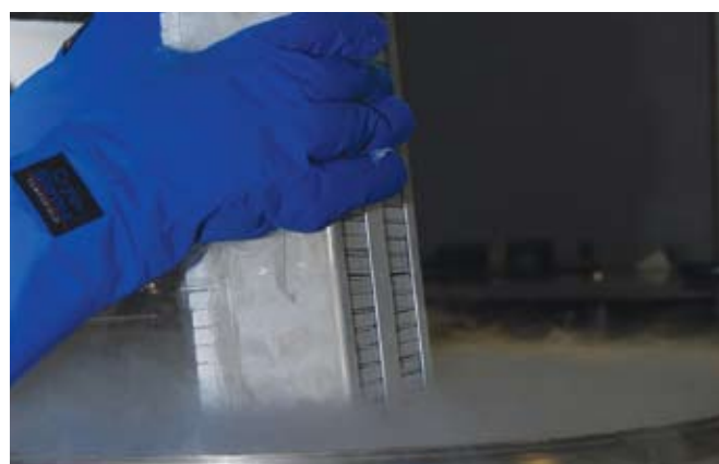
Stem cells packed in canisters safely stored in gas phase of liquid nitrogen.
