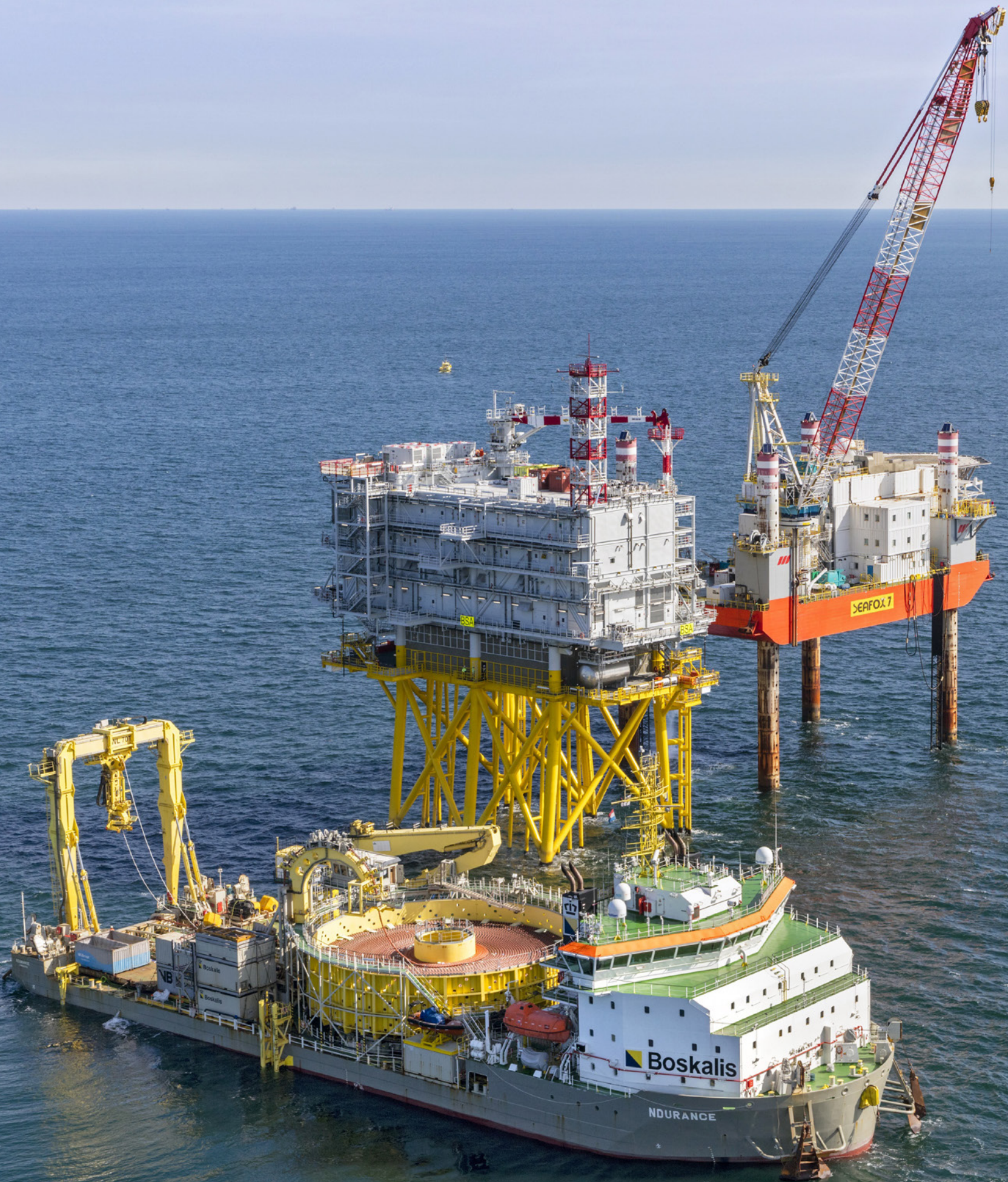
Cable-laying vessel Ndurance installing power cables as part of the Borssele Alpha project
