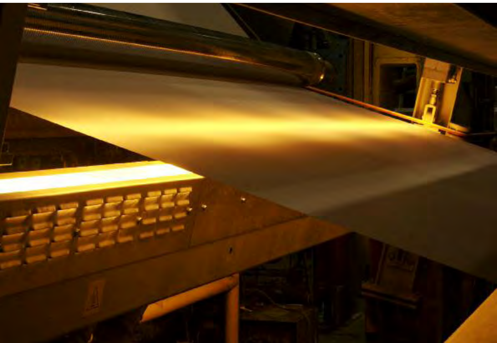
Web inspection system for online visual quality control of the paper.
