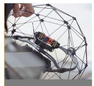
to inspect tank walls. The 'Elios' drone is specially designed to move in small spaces where it can bump into the walls without damaging the object or the drone. The drone is used to inspect the space between the inside of the gas tanks at the terminal.
