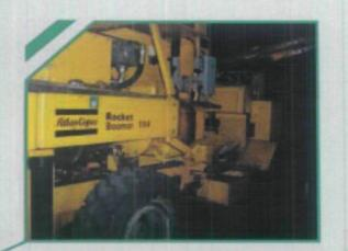
Drilling by drilling Jumbo Boomer 104
