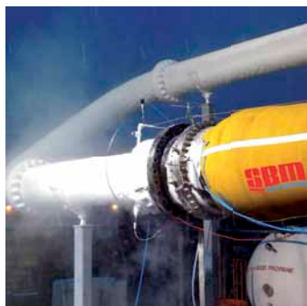
Top: Image from the PDMS model showing a disconnectable turret for arctic application Middle: COOL™ LNG hose during line test with LNG Bottom: Image from the PDMS model showing the disconnectable turret for FPSO Okha
