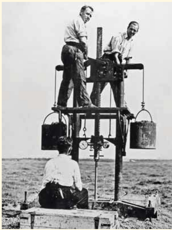
First manually operated cone penetration test (1945).
